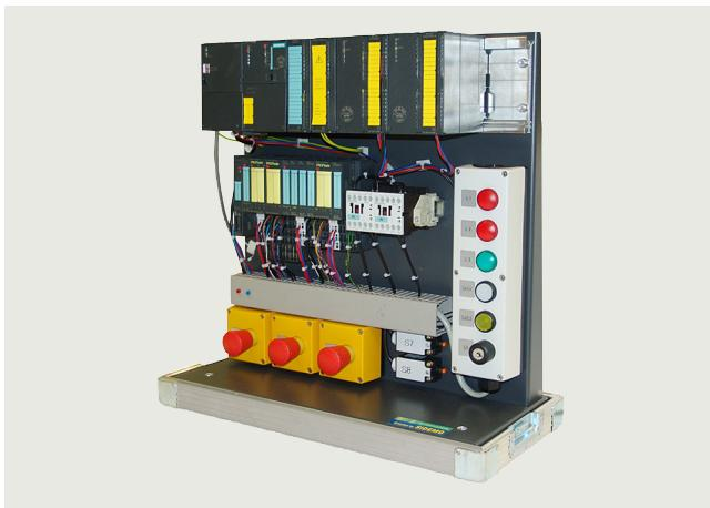
The training case is used to realistically practice the programming, operating and commissioning of fault-tolerant S7-300 controllers.
