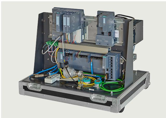
Standard training equipment for the SIMATIC PCS 7 course portfolio. The transportable case can be combined with any automation system with a PROFIBUS DP interface.
