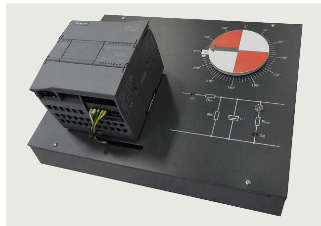
The training module is used to work with the Technology Functions (Motion Control Axis and PID Loop Control) of the SIMATIC S7-1200 in realistically practice exercises. It serves as an extension of the SIMATIC S7-1200 and SIMATIC S7-1500 training devices.
